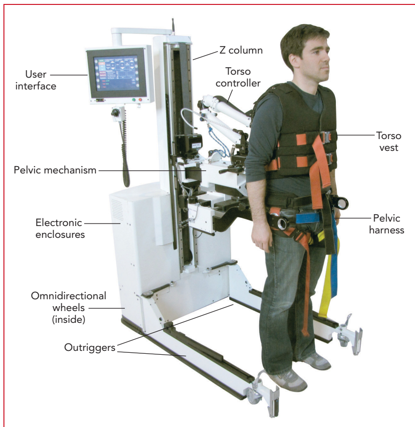
FIGURE 1. In the KineAssist system, control algorithms move the motorized base in response to the patient's own forces and motions. Courtesy of Kinea Design.
