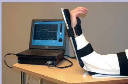
By measuring minute force outputs, QMAD helps physicians determine whether surgical or pharmacological interventions are helping a patient regain muscle strength and motion. Courtesy of Kinea Design.
